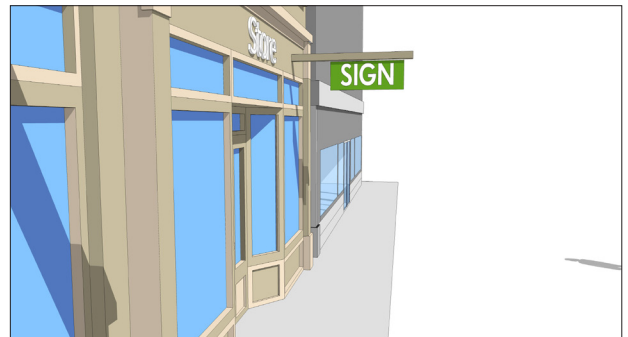
A typical projecting sign
